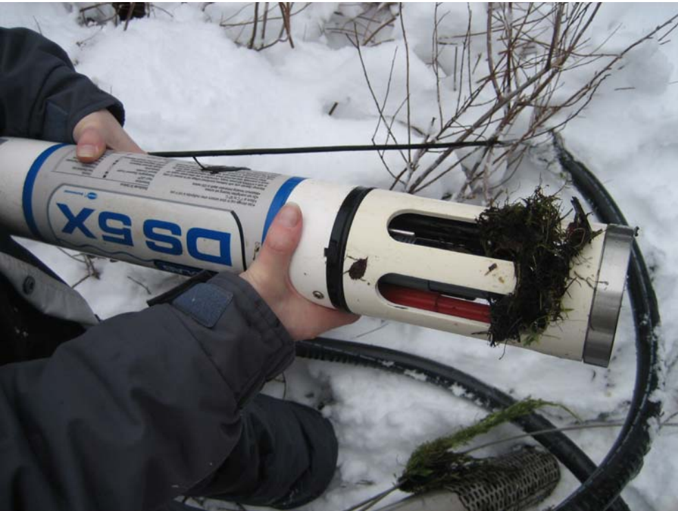
Picture 3: Alga/plant material that was found intertwined on the Datasonde when instrument was removed on January 23 rd , 2007
