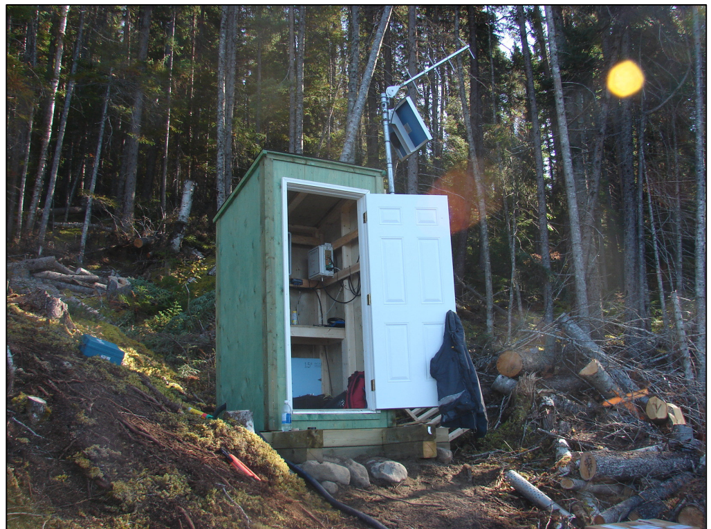
Figure A-4: Photograph of protective hut at RTWQ station below Metchin River. Data logger (white box) inside the hut is also visible
